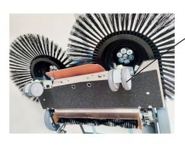
(1) Check drop function - swivel caster must be move easily, remove any material or dirt caught in the wheels.
