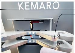
**(4)** Clean charging contacts on the robot and charging station with a cloth.
