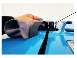
(2) Clean LiDAR with compressed air or a soft lint-free or microfiber cloth.
